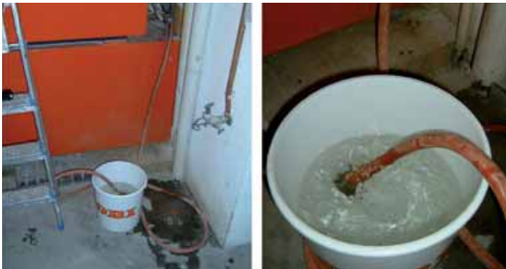
Heating water sample 26.06.2008 The heating water has become clear after approximately 7 weeks
